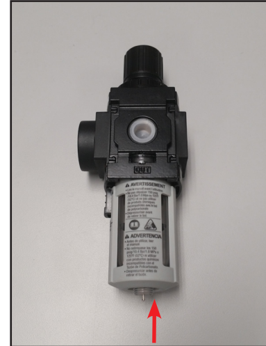
Fig. 1: Draining accumulated water in air filter
