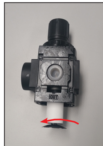
Fig. 3: Replacing air filter
