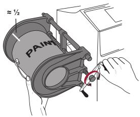
3. If mixing with only one clamp on a Model 1400, install an empty can (or a piece of 2" x 4" board) in the other clamp.
