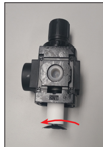
Fig. 3: Replacing air filter
